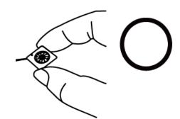
Don't pull fan with lead wires.
